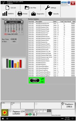
Inbuilt machine statistics page with preventative maintenance warning system
